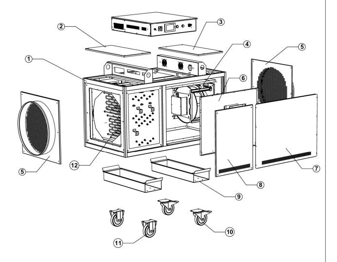
Model Alfa-Jet 100 kW Industrial Type Electric Fan Heater
